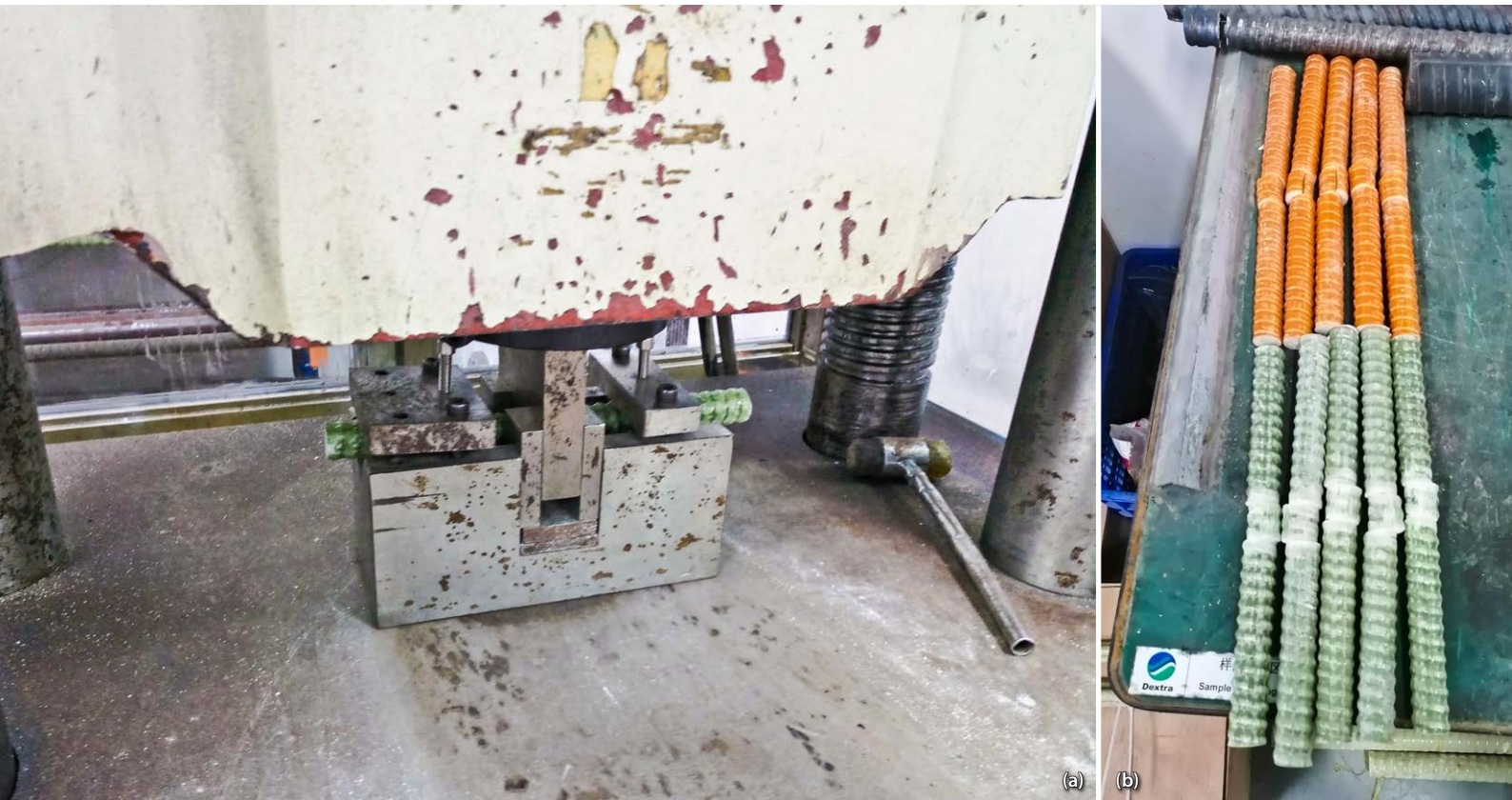
Figure 7 Double shear test on GFRP bar
