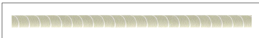
Figure 2 Dextra GFRP rebar with FRP fibres wrapped around the longitudinal bar together with sand coating to enhance bond strength
